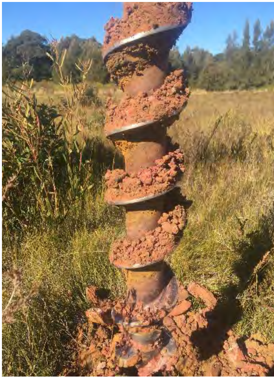
Photograph 16: Residual to extremely weathered material encountered at 1.5m depth typically found in test locations across the site.
